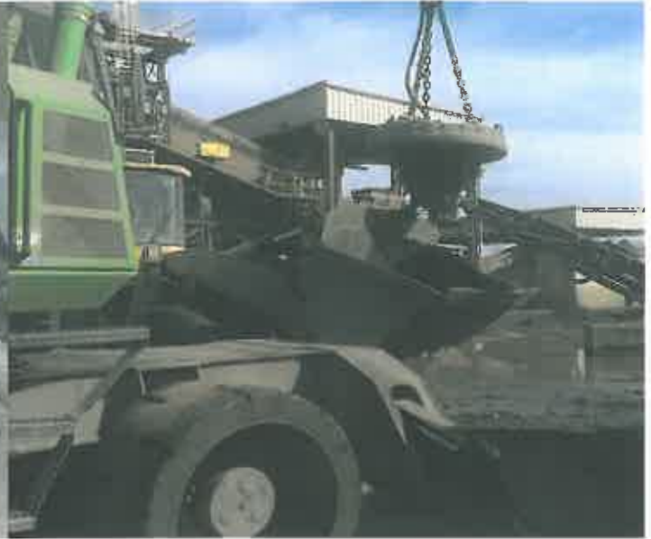
Figure 3.3 Experiment to remove metal (shows metal from one bucket load of material).
