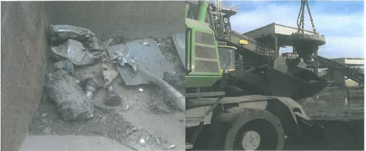
Figure 3.2 Examples of metal contamination present in the auto fluff. The shovel head is present for size comparison.
