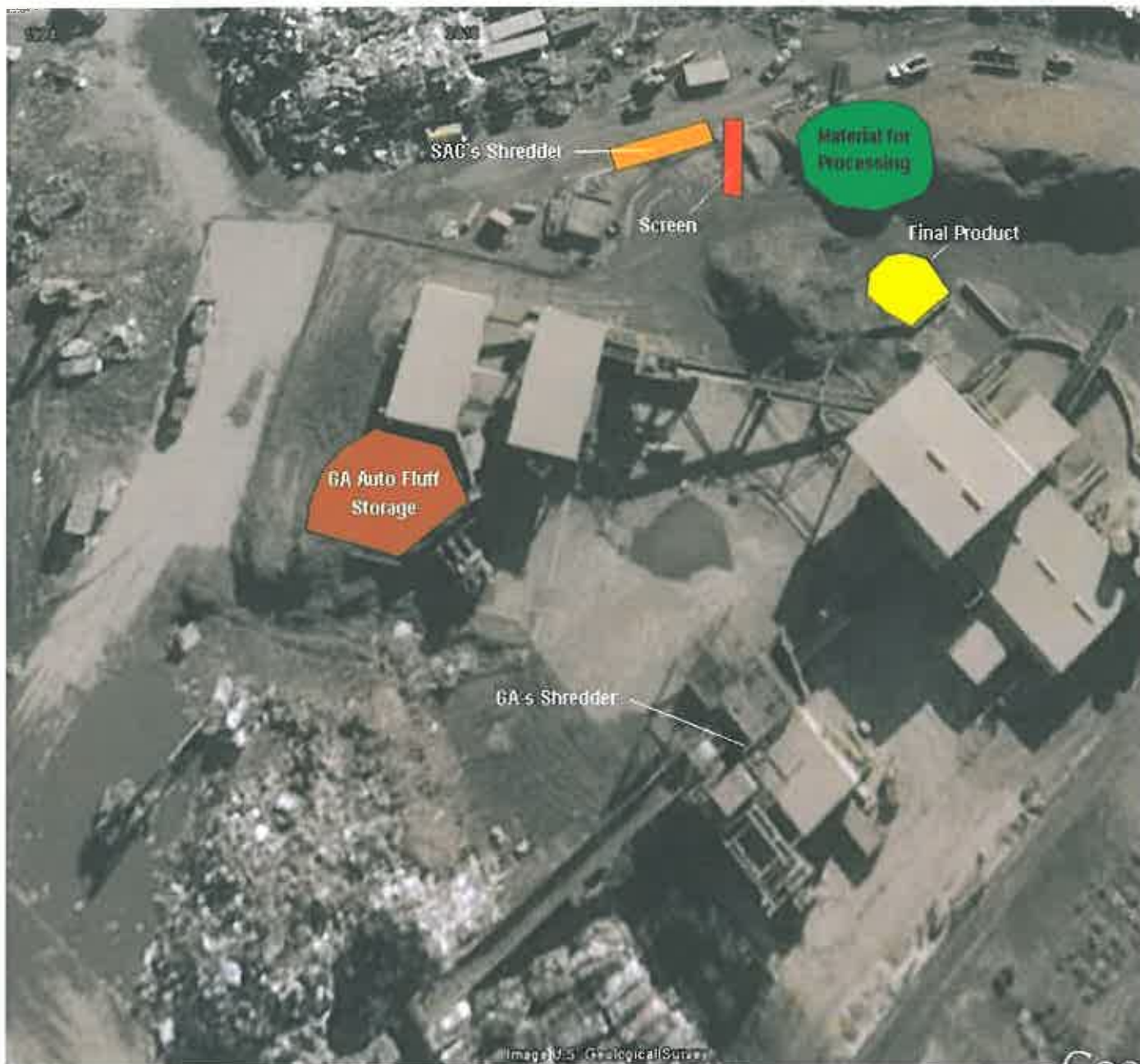
Figure 3.7 Aerial view of GA shredder operations with diagrams showing the location of SAC's re-shredding operations.
