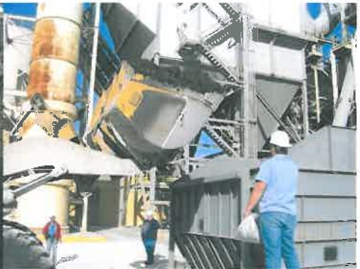
Figure 2.5 Experiment to remove metal (shows metal from one bucket load of material).
